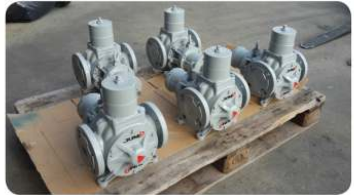
JV15c bare shaft pumps
